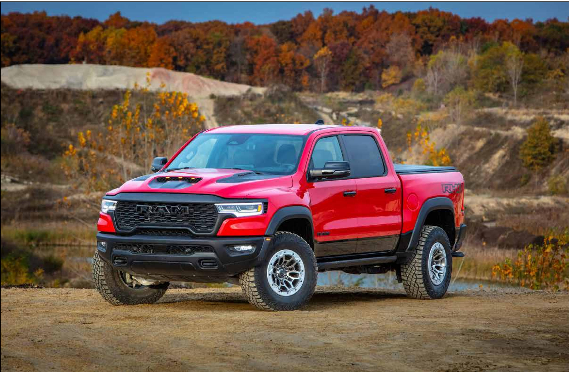
The 2025 Ram 1500 RHO stands eight inches wider than standard Ram trucks, with composite fender flares housing 35-inch tires on optional 18-inch bead-lock capable wheels.
