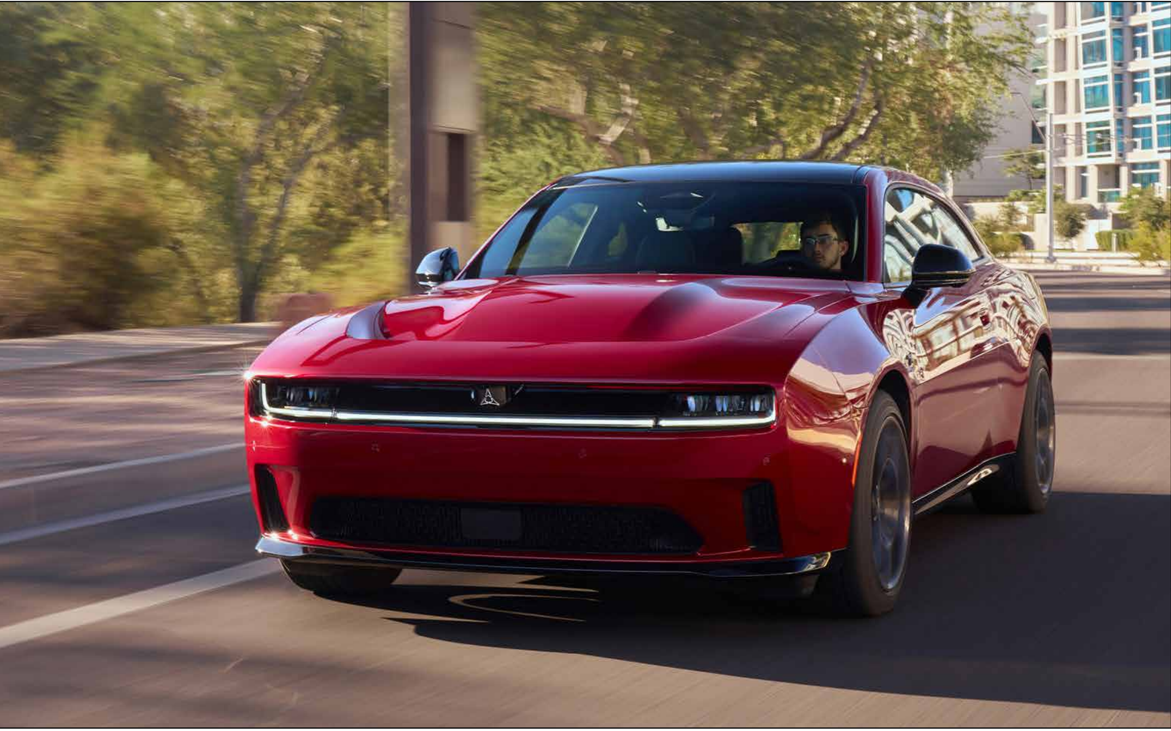
The Dodge Charger Daytona R/T features the innovative R-Wing front design that allows air to pass through the nose of the car, combining retro muscle car styling with functional aerodynamic benefits.
