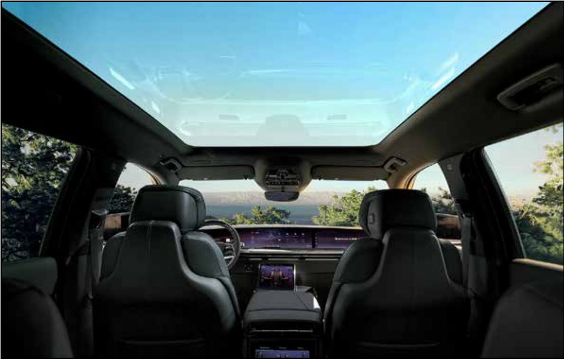
The Escalade IQL’s cabin includes a curved 55-inch display spanning the dashboard and an optional Executive Second Row package with personal screens and dedicated amenities.
