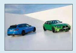
**M3, M3 TOURING** The 3.0-liter twin-turbocharged straight-six now has 530HP, a 20HP increase. BMW tweaked the headlights with arrow-shaped LEDs, too.
